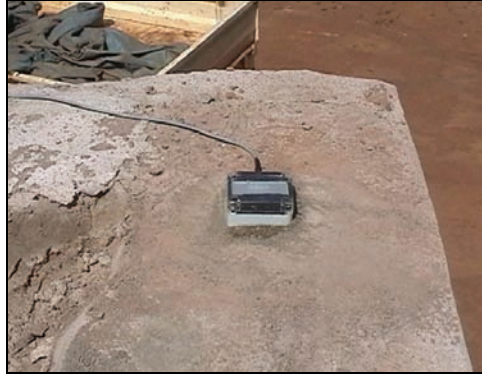
Figure 11: Irradiation meter on the roof of the LESCO office.
